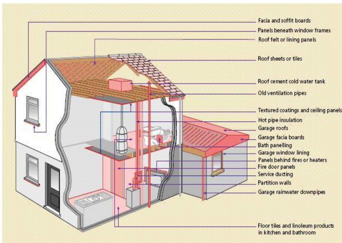
ACMs might be found in roofs, claddings, soffits, window cills, bath panels, chimneys/flues, water tanks, floor tiles and textured coatings (Artex or similar). As you can see above there are many products, but this list is not exhaustive.
