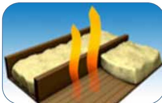
4.10.2. It is important to ventilate the roof space, above the insulation, in order to reduce the risk of condensation. If the roof space is to be used for storage, bearer boards should be placed across the existing joists, to prevent the insulation from being compressed.
