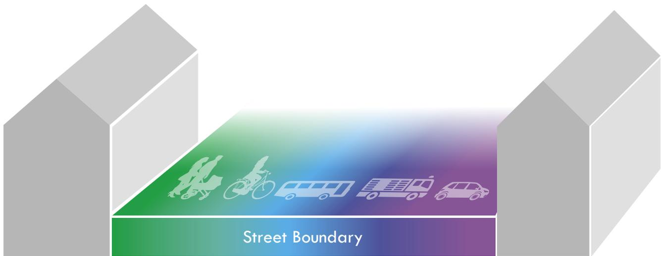
*When allocating dimensions for road boundaries a number of criteria need to be considered, which includes both vehicular and non-vehicular/pedestrian demands; current and potential future requirements of the infrastructure and the impact different drainage methods would have on the design.*
