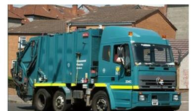
Access roads should be built to withstand a gross vehicle weight of 32 tonnes with an axle loading weight of 11.5 tonnes. The turning circle requirement should be in the region of 24 metres or a suitable swept path hammer head detail. Refuse collection vehicles should not be expected to carry out a lengthy reverse manoeuvre if at all possible.
