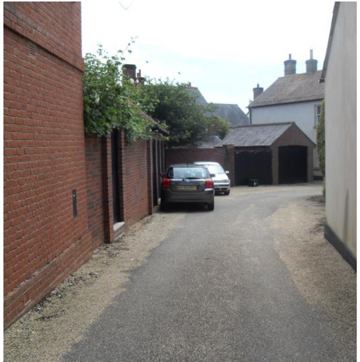
Shared surfaces can lead to indiscriminate parking, blocking of footway and the narrowing of the road which hampers access by service and emergency vehicles. Shared Surfaces should therefore only be used in appropriate circumstances, at very low densities.
