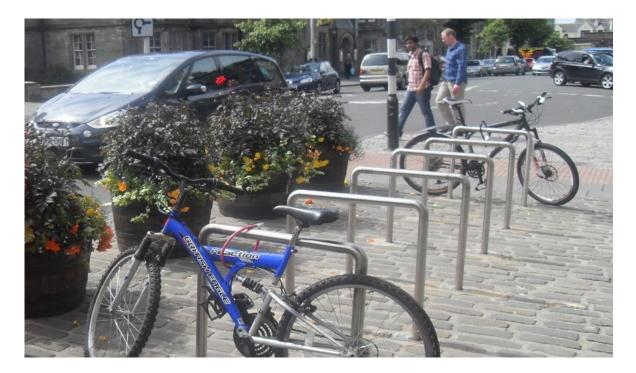
Normally Sheffield stands should be provided. Stands that grip only the front wheel do not provide adequate support or security. When placed 1 m apart and 0.5 m from the wall, Sheffield stands can accommodate two cycles. Where more than two stands are required, you may need to provide a 'toast rack' facility.
